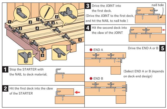
X Standard number of the NAIL used: 1 for the JOINT, 1 for the STARTER, 2 for the END
