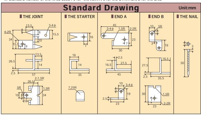
■ Standard number used in case two-by-four wood (38mm x 89mm), 60cm between joists
