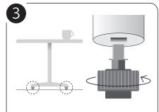
Mount the T.balance with the attached adapter to the internal threads of the table leg.
