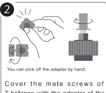
Cover the male screws of T.balance with the adapter of the correct size and attach it.
